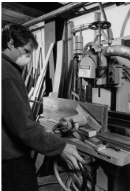
Whit McLeod uses a vintage chain mortiser to prepare a piece for joining.
